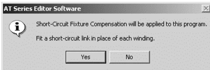
At this point you should ensure that the appropriate fixture has been placed on the tester and a short-circuit bobbin fitted. For the following open-circuit compensation, remember to remove the short-circuit bobbin.
