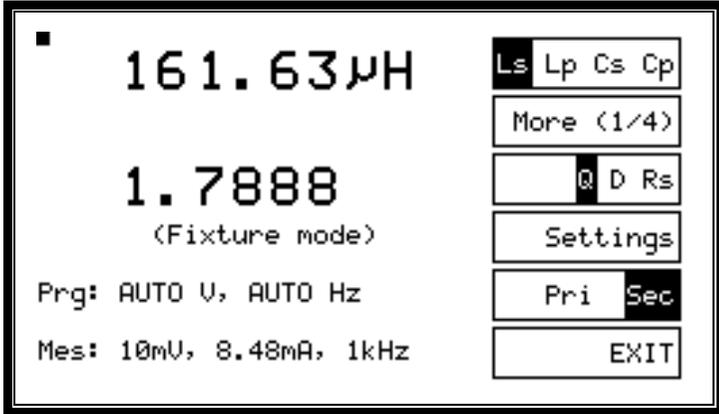
For measurements of TR (turns ratio) and TRL (turns ratio by inductance), softkey 5 toggles the display of measured test conditions. It does NOT alter the designation of primary (13,15) and secondary (14,16). Turns ratio is always displayed as the ratio between primary (13,15) and secondary (14,16) windings.
