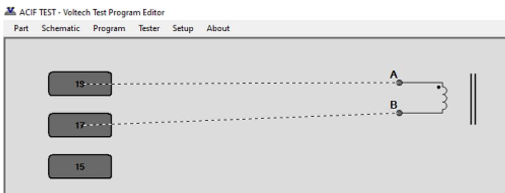
4, Add a VOCX test, with the same 19/A and 17/B nodes used for BOTH Energised and Measured terminals
