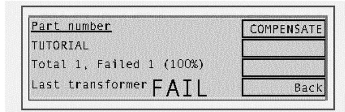
Press COMPENSATE to repeat the fixture compensation measurements, or 'Back' to return to the RUN-FINISH display without re-compensating.
