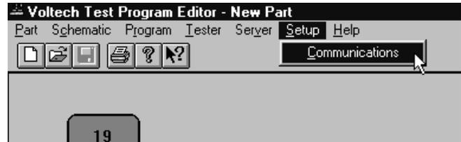
2. In the dialogue box shown here; select the PC communications port which is connected to the tester.
