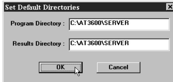
The setting of storage path directories may be altered at any time. The directory setup dialogue may be found under the SETUP section of the menu bar.
