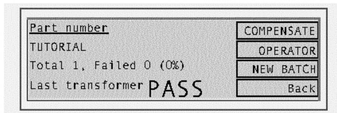
To change the operator name, press the OPERATOR soft-key.
