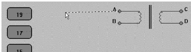
To change a connection, simply use the right button to pick it up and move it to either another test node or to another transformer terminal.
