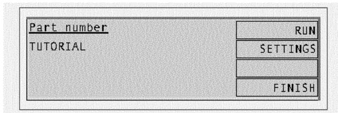
Place the component to be tested in the fixture and press the RUN soft-key, or the footswitch.
