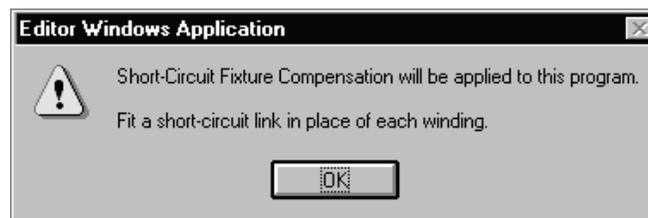
At this point you should ensure that the appropriate fixture has been placed on the tester. With the first message, it is possible to leave the fixture empty.
