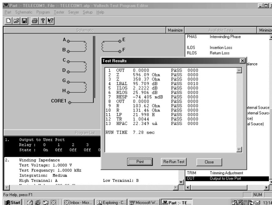
If you look at the test results screen shown above, you will see that test 4 (LBAL) contains a status error code of 0010. This error code indicates that “The measurement had not settled in time”. Although this test passed, it indicates that a problem existed during the test sequence. In this particular example, the fault was due to a poor connection to the core of the transformer.
