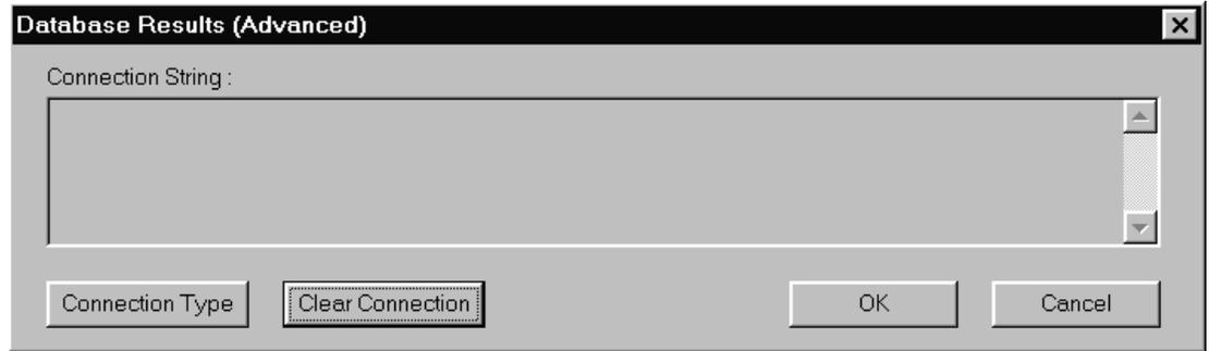
To connect to your database, the Server software uses a connection string that contains (amongst other things) the name of a provider, the name and location of the database and a valid database user name and password (if required). You may need to consult with the database or network administrator to obtain this information.
