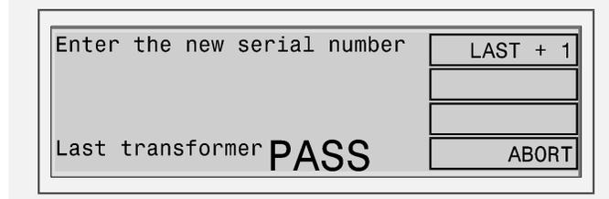
If the next serial to be used simply follows on in sequence after the previous one, then press the LAST + 1 soft-key (or the footswitch). This will enter the next serial number automatically and return the display to the RUN-FINISH selection.
