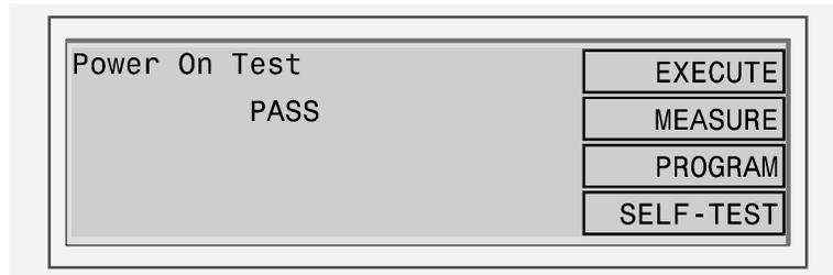
The tester is now at the Top Level menu, and the soft-keys allow you to select which of the four main functions you require:
