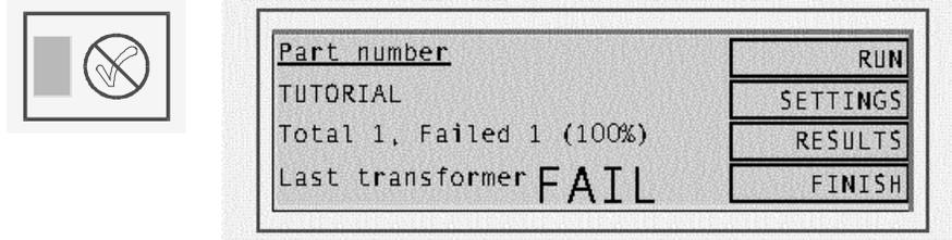
The RUN-FINISH displays seen after a previous component has been tested.
