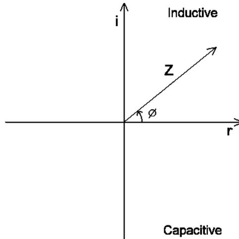
The impedance phase angle test measures the angle  $\phi$  of the impedance vector  $Z$ , as shown in the phasor diagram. It represents the phase difference between the fundamental current flowing through a winding and the fundamental voltage across it. This test is normally used for audio and telecommunication transformers along with the  $Z$  test to check the complex impedance presented to the transformers input and output.
