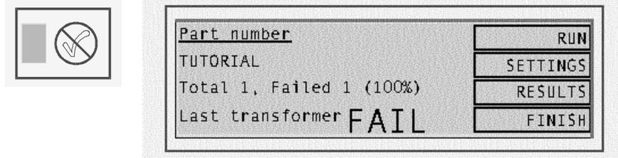
If you think that fixture compensation needs to be re-measured at any time, at the RUN-FINISH display, press the 'SEETINGS' soft-key to reveal:
