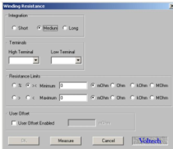
Initially enter the terminal names. Input 'A' as the high terminal and 'B' as the low terminal, moving between the fill-in boxes using the TAB key.
