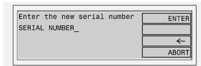
After typing the new number, press the ENTER key, the ENTER soft-key or the footswitch to return to the RUN finish display.
