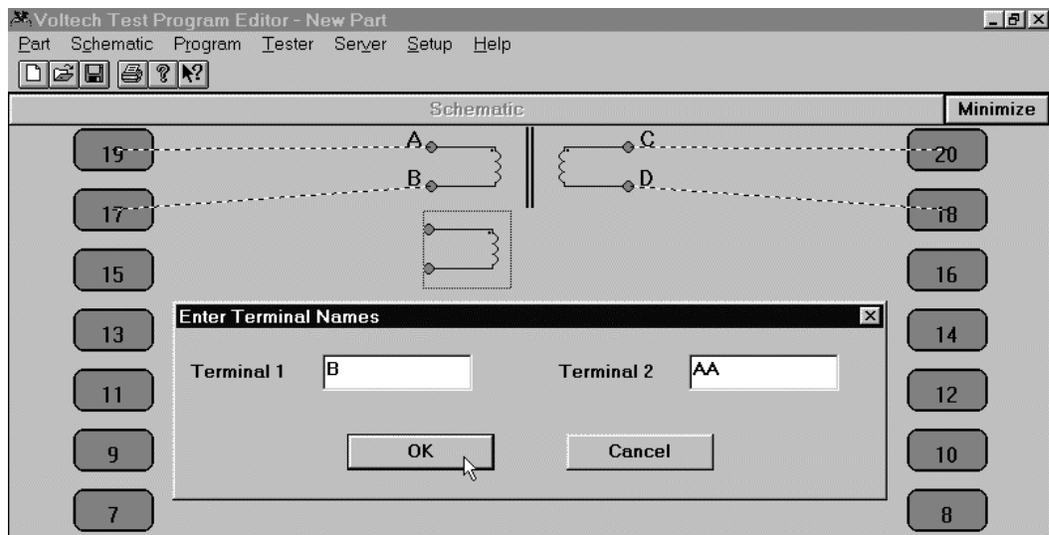
Upon clicking the left mouse button, a form fill-in dialogue box will appear on the screen with prompts to insert the terminal names of the new winding.
