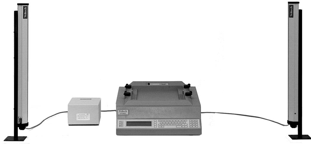
The light curtain is positioned in front of the tester. It extends well beyond the width of the tester so that the operator is not impeded when he/she has to load and unload the transformer under test.
