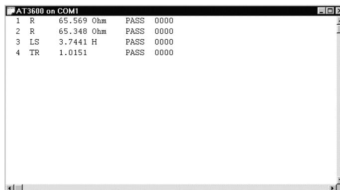
Test results may also be reviewed at any time via the tester's front-panel results listing screen, which is accessible from the RUN-FINISH display by pressing the RESULTS soft-key.
