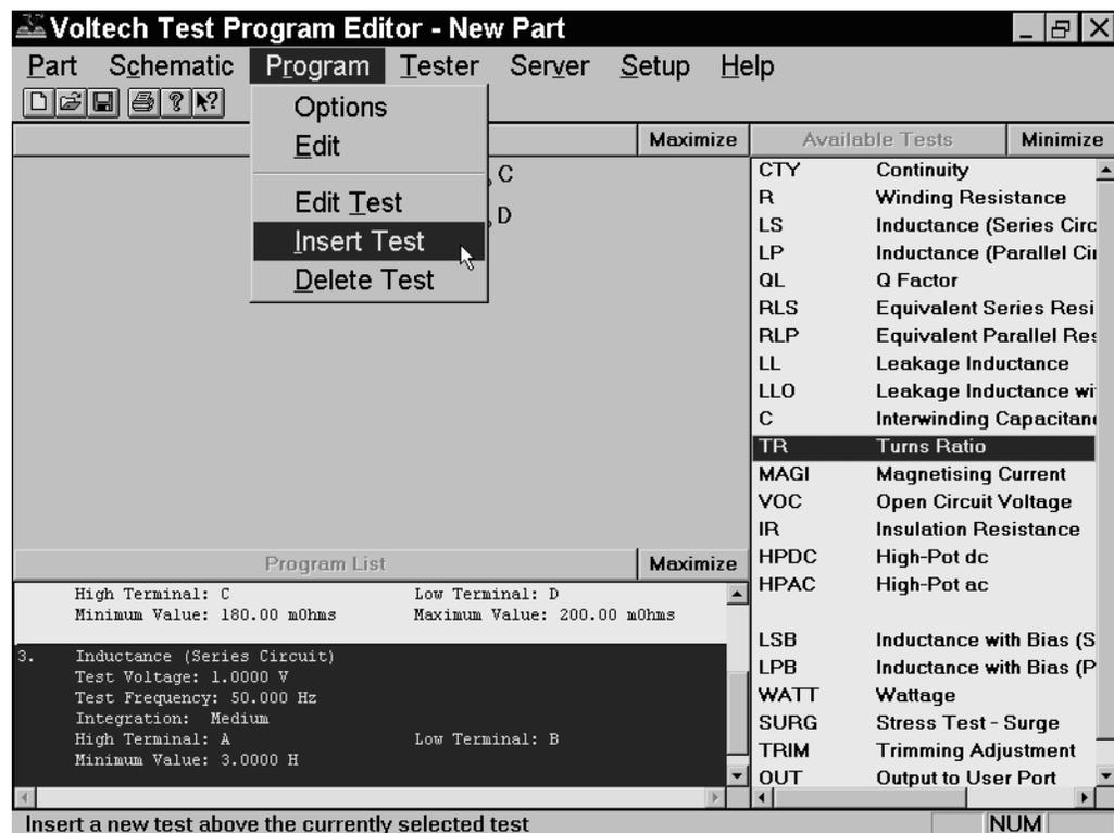
In this example, a Turns Ratio test will be inserted before the Inductance test 3 in the Program.
