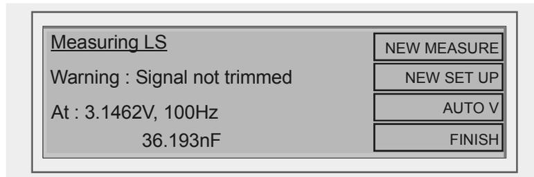
The AT will continue to measure accurately, but you can also allow the tester to automatically choose a test voltage or current based on the programmed frequency by selecting AUTO V.
