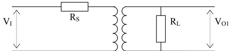
The resistors shown are fitted to the test fixture and should be switched out of circuit when making other measurements such as resistance and inductance. This can be done by fitting relays to the fixture and switching them at appropriate points in the test program using OUT tests.
