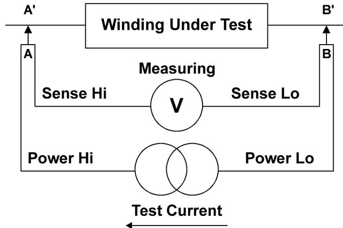
The AT series testers provide all the connections required to take advantage of Kelvin measurements.
