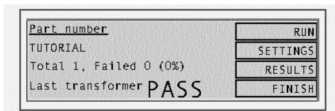
Before running any new test program, return the tester to the top-level menu by pressing the FINISH soft-key (i.e. the 2nd soft-key from the top).
