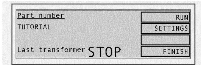
The RUN-FINISH display seen after measurement of the previous component was halted using the STOP soft-key, or the STOP input of the remote port.
