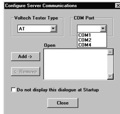
A check box 'Do not display this dialogue at Startup' exists to prevent it from being displayed each time the Server application is launched. When this option is activated, this dialogue box can be accessed via the 'Setup', 'Communications...' menu.
