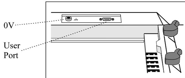
The port contains six open-collector relay drive outputs, and two HC MOS compatible inputs.
