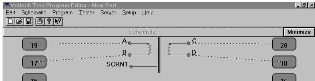
A connection from the screen will appear on the schematic. You may now add a screen-to-node connection.
