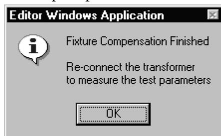
After you have clicked on the 'OK' button, the tester will be commanded to make its measurements, and you will see the following message:
