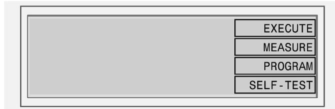
To access PROGRAM Mode, from the top level menu, press the soft-key PROGRAM to change to the following display:
