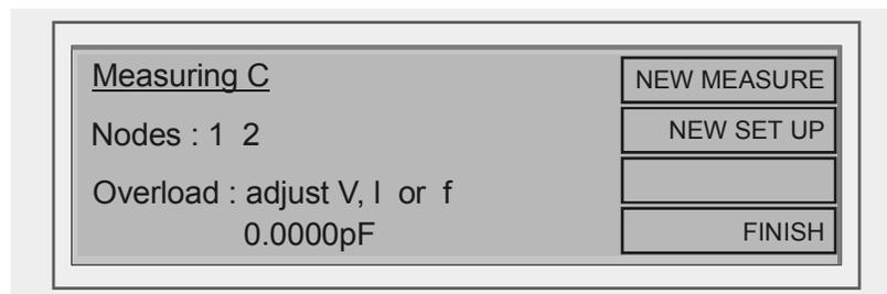
In this case, choose AUTO conditions where possible in a NEW SET UP and consult Chapter 7, Tests and Test Conditions. For low voltage / low power tests only, the tester will continue to try making measurements.
