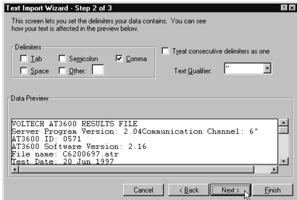
In the 'Delimiters' section of this screen, ensure that only the 'Comma' option is checked. Click on 'Next >' and proceed to step three:
