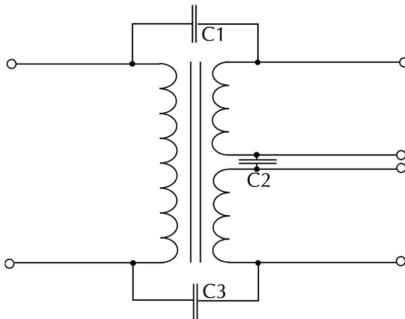
Inter-winding capacitance may be of interest in transformers used in audio, medical and instrumentation applications, where isolation between primary and secondary windings is important. It can also play an important part in the circuit operation of switch-mode transformers where, for example, too large a capacitance may give rise to a large amount of noise at the switching frequency being coupled into sensitive circuits connected to the secondary windings.
