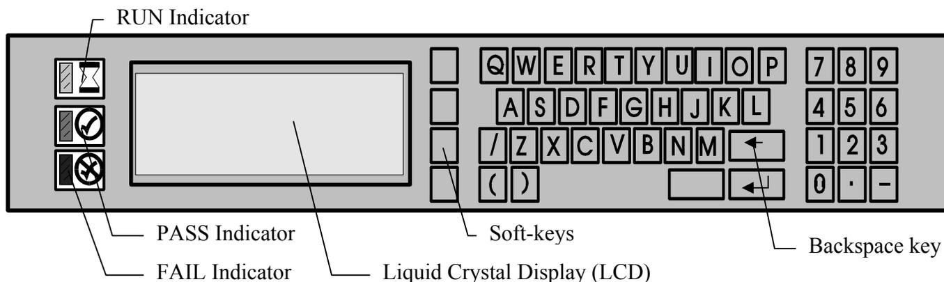
The front panel of the AT Series testers is designed with a membrane type keyboard and liquid crystal display. The main features are as follows:
