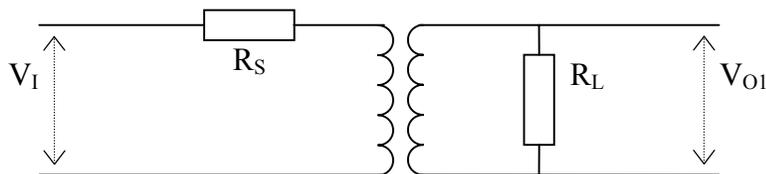
$$ILOS = 10 \log (V_I^2 R_L / 4 V_{O1}^2 R_S)$$
