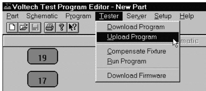
This will transfer the current program from the editor to the server. The program will be sent via the tester's serial link if present, by direct file transfer if both applications are resident on the same PC or by network file transfer if a network link is present and is identified to the server.
