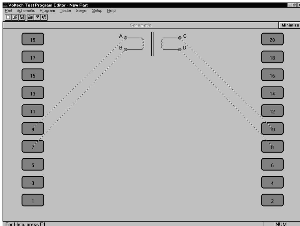
You have now created a schematic layout of a four terminal transformer.
