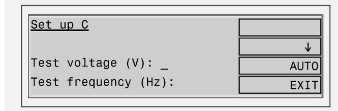
The details of the set up display will vary depending on which test you have selected. For the capacitance test, the list of parameters to enter is: Test voltage, Test frequency, Integration, Hi node(s), and Lo node(s). For Winding Resistance, the list is simply: Integration, Hi node, and Lo node.
