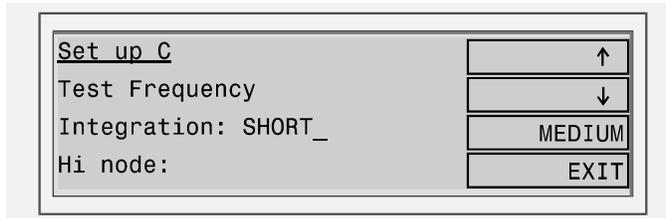
Because node numbers (1 to 20) are used in the MEASURE Mode, the test nodes are entered using the keyboard number pad. After each node number has been typed, proceed to the next by using the cursor (↑ or ↓) soft-keys, or by using the ENTER key (↵).
