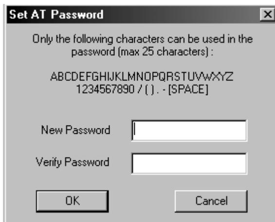
Note that this Editor dialogue also allows the password to be reset. The old password is not required to do this. All that is required is for the new password to be entered and verified.
