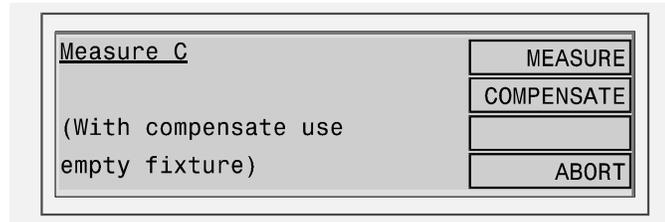
If you wish to apply Fixture Compensation to the measurements, ensure that the fixture is empty, and press the COMPENSATE soft-key. When the Compensation is finished, the display will return to one similar to the one above, but with the COMPENSATE soft-key and message omitted. (For some tests there is no COMPENSATE option, and for others compensation requires the fixture to be fitted with short-circuit links.)
