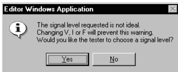
Check first that the winding is properly connected to the right nodes. Choose 'Yes' and the AT will choose suitable voltage conditions for you and enter them into the test dialogue. Choose 'No' and no conditions will be chosen. See Chapter 7 – Tests and test conditions for suitable values.
