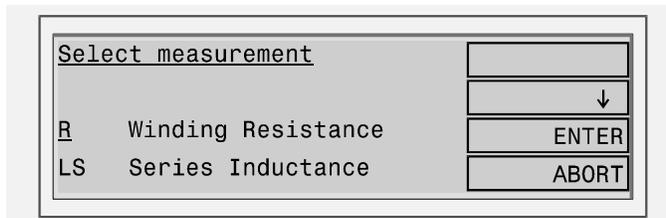
By using the soft-key cursors ( $\uparrow$  and  $\downarrow$ ) or by typing the initial letter of a test, you may select the test you require. The cursors are displayed only when they are valid, hence the  $\uparrow$  cursor is not visible when the screen is displaying the top line of the list of tests.
