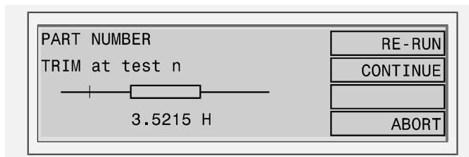
The main difference between this and the 'Stop on fail' display is that the reading on the fourth line will be continuously updated, allowing adjustments to be made to bring the test result within limits.
