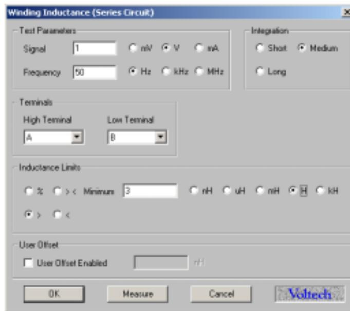
The "User Offset Enabled" check box has the same function as before but in units of inductance.
