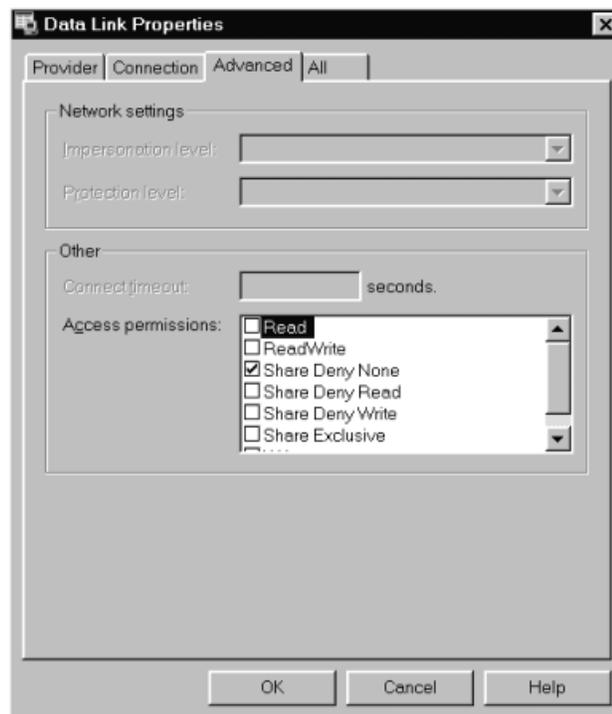
Check that the 'Access permissions' for the database are as required. 'Share Deny None' is the default and is usually the most suitable setting.
