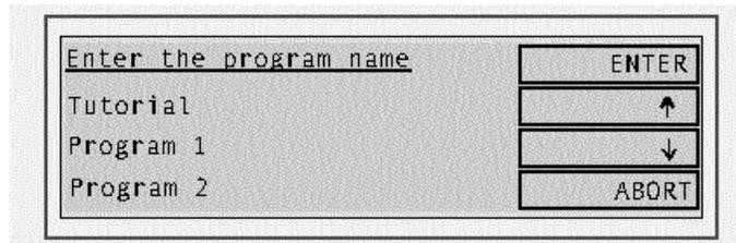
If the list of programs fails to appear after a few seconds, check that the server is running and that the COM port and file folder are correctly configured. Is the cable from the AT3600's server port to the PC fitted correctly?
