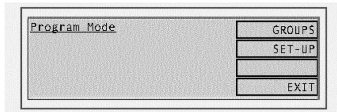
The two main functions of PROGRAM mode each have their own soft-keys at this display. Press the GROUPS soft-key to download a group of test programs from the server to the tester's internal memory or press the SET-UP soft-key to change any of the set-up options.
