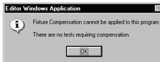
When you click on 'OK' to return to the top level menu, the tester will not make any measurements.
