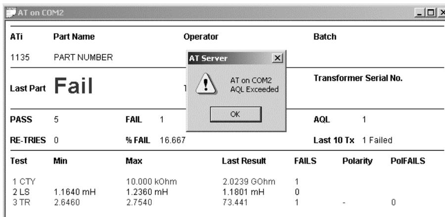
Click on 'OK' to acknowledge the warning. You will be given the option to disable the warning for further parts in the batch. Normally, you would select 'No' to leave the AQL checking active for the rest of the batch. When a new batch is started, the AQL level is reset according to the level entered for the part using the Voltech AT Editor.
