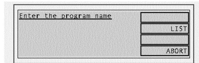
The program name can now be typed at the keyboard, entered by swiping a barcode or chosen from a list. Press the soft-key LIST to see a list of the programs available on the PC server or in the AT3600's own memory (see section 6.6.2)
