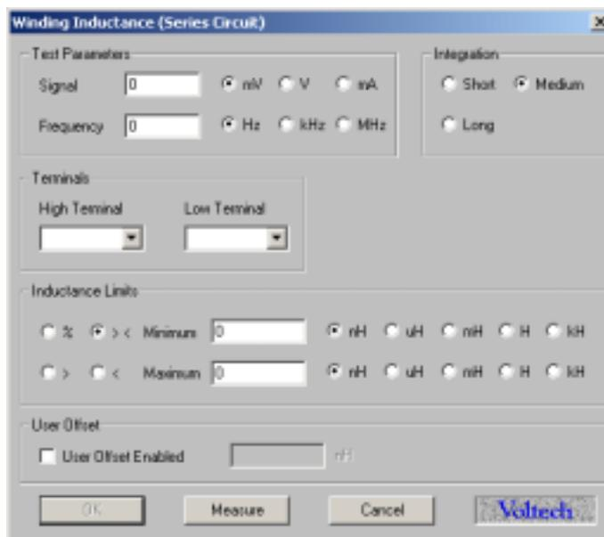
For many tests, including the LS test, you may enter the Test Parameters in two ways: either by simply keying in the numbers you require, or by using the Measure button.
