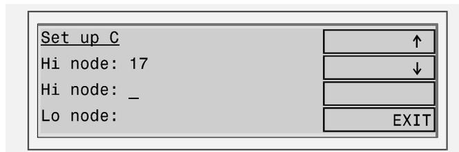
As you enter more numbers, these will be added to the list of Hi nodes. When you press the Enter key, or the ↓ soft-key with no new number (for example at the display above), then the group of Hi nodes will be terminated, and the display will move to the Lo nodes:
