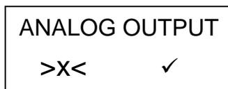
If this menu is not available, turn off the power, disconnect the power lead and any other leads, and check that the Interface has been correctly plugged in. On continued failure, contact your Voltech distributor.
