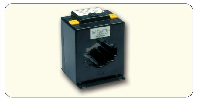
The Voltech CT1000 is a toroidally wound AC current transformer that extends the range of Voltech power analyzers such as the PM100, PM300 or PM3000A to 1200A rms. Close- tolerance current ratios provide a measurement accuracy of better than 0.2%, making the CT1000 suitable for precision-grade measurements.
