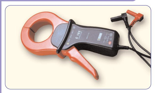
The Voltech CL1000 is a clamp-on current transformer that extends the AC current capability of Voltech power analyzers such as the PM100, PM300 or PM3000A to 1000A rms.
