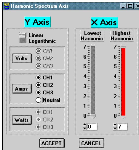
In this box the user can select the type of Y axis (linear or logarithmic), the parameter of the Y axis along with the channels to be displayed and the range of harmonics. While in Logarithmic mode, the zooming and panning of the Y axis is disabled.
