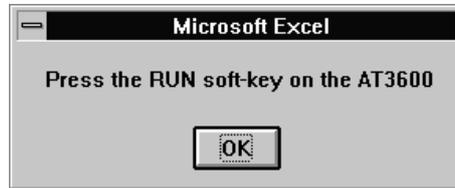
Click on the OK button. When you have pressed the RUN soft-key and the first result has been read, the message box will disappear, and you will then see the first result entered into cell F3 of the spreadsheet.
