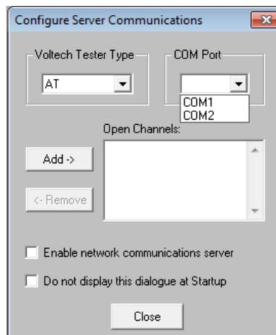
Select a COM port that is connected to the server port of an AT series tester, and then click the Add button to add this AT to the list of open channels as shown
