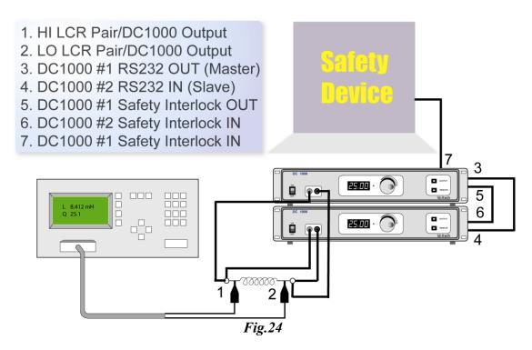
Please take care not to insert the safety interlock cable into the RS232 port on the rear of the DC1000. Doing so could damage your instrument.
