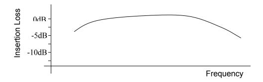
The RESP test consists of a number of Insertion Loss (ILOS) tests repeated at different frequencies.
