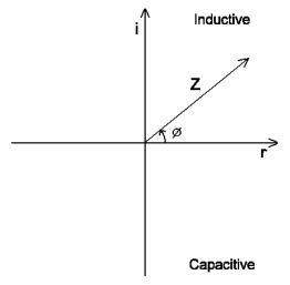
The impedance phase angle test measures the angle  $\varnothing$  of the impedance vector Z, as shown in the phasor diagram. It represents the phase difference between the fundamental current flowing through a winding and the fundamental voltage across it. This test is normally used for audio and telecommunication transformers along with the Z test to check the complex impedance presented to the transformers input and output.
