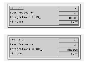
Because node numbers (1 to 20) are used in the MEASURE Mode, the test nodes are entered using the keyboard number pad. After each node number has been typed, proceed to the next by using the cursor ( $\uparrow$  or  $\downarrow$ ) soft-keys, or by using the ENTER key ( $\downarrow$ ).
