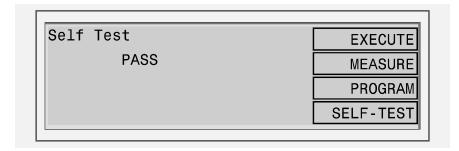
To ensure operator safety, the high voltage sources are not checked until about 10 seconds after the start of self-test.
