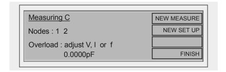
In this case, choose AUTO conditions where possible in a NEW SET UP and consult Chapter 7, Tests and Test Conditions. For low voltage / low power tests only, the tester will continue to try making measurements.
