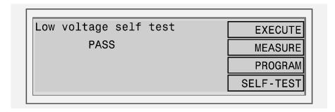
Without a safety interlock system the unit cannot perform any high voltage self tests, hence the high voltage sources are disabled.
