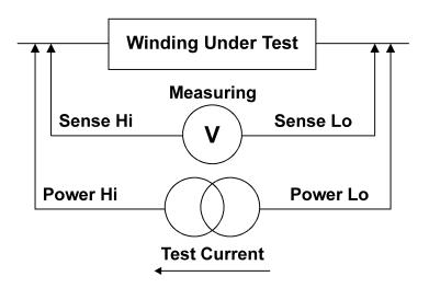
In this arrangement, the test current passes through the two 'power' leads, and the voltage is measured using the two 'sense' leads.
