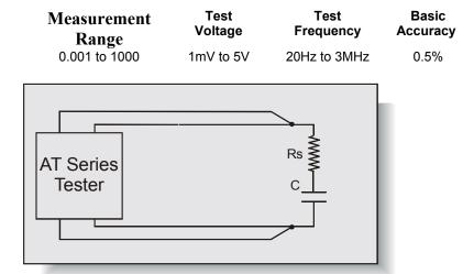
The parameter 'D' is most often used as a measurement of the losses in a capacitor. It is analogous to Q for a transformer winding.
