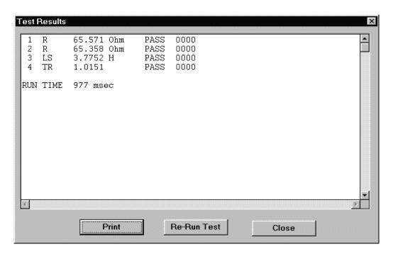
If no transformer is fitted, the results will have no meaning, but **you have now** successfully installed the AT3600 and the Voltech AT editor software.
