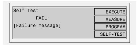
The message shown on the lower two display lines will depend on what caused the failure.
