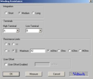
Many of the tests available for the AT Series have all four limit types. There are obviously some tests where it is not sensible to have four limits, IR - Insulation Resistance - being a clear example where only a minimum limit is applicable, as the perfect insulation between windings has no upper limit to its resistance.
