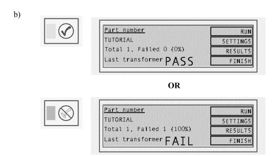
The RUN-FINISH displays seen after a previous component has been tested.
