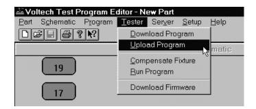
This will transfer the current program from the editor to the server. The program will be sent via the tester's serial link if present, by direct file transfer if both applications are resident on the same PC or by network file transfer if a network link is present and is identified to the server.
