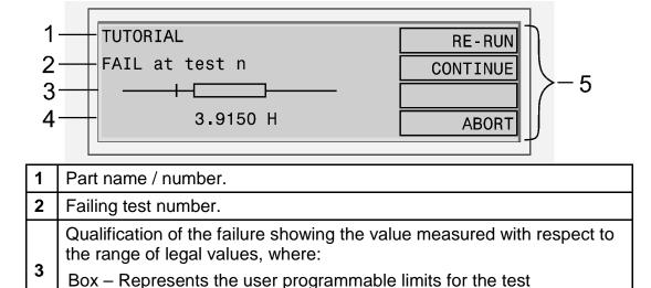
From this display, after you have pressed the CONTINUE soft-key, the tester will execute the remaining tests in the program, and the transformer will be recorded as a fail. (If any further tests fail, then there will be another display similar to the one above for each failing test.)
