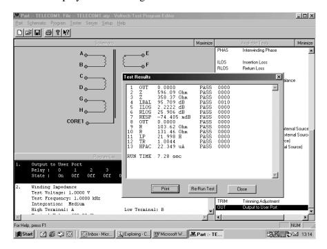
If you look at the test results screen shown above, you will see that test 4 (LBAL) contains a status error code of 0010. This error code indicates that "The measurement had not settled in time". Although this test passed, it indicates that a problem existed during the test sequence. In this particular example, the fault was due to a poor connection to the core of the transformer.
