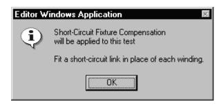
Fit the required short-circuit header, and click on 'OK'.
