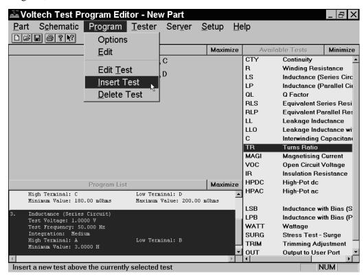
In this example, a Turns Ratio test will be inserted before the Inductance test 3 in the Program.
