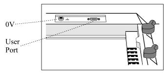
The port contains six open-collector relay drive outputs, and two HC MOS compatible inputs.
