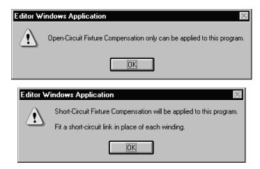
At this point you should ensure that the appropriate fixture has been placed on the tester. With the first message, it is possible to leave the fixture empty.
