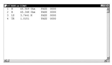
Test results may also be reviewed at any time via the tester's front-panel results listing screen, which is accessible from the RUN-FINISH display by pressing the RESULTS soft-key.
