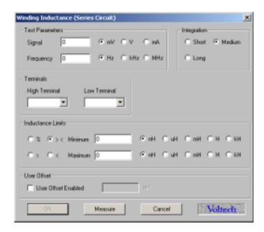
For many tests, including the LS test, you may enter the Test Parameters in two ways: either by simply keying in the numbers you require, or by using the Measure button.
