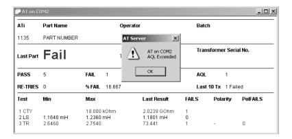
Click on 'OK' to acknowledge the warning. You will be given the option to disable the warning for further parts in the batch. Normally, you would select 'No' to leave the AQL checking active for the rest of the batch. When a new batch is started, the AQL level is reset according to the level entered for the part using the Voltech AT Editor.
