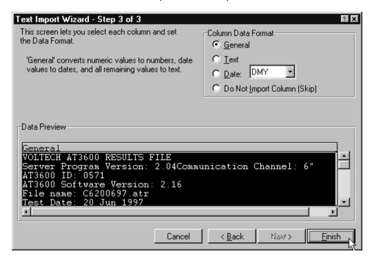
Check that the 'Column Data Format' option is checked as 'General' and click on finish.
