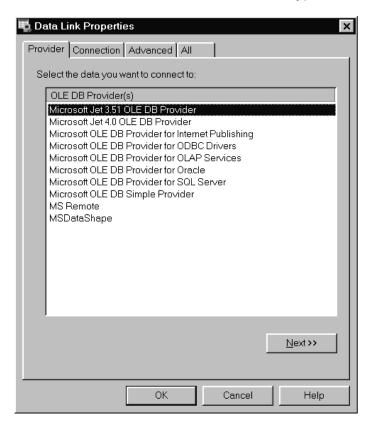
The 'Data Link Properties' dialogue is a standard one that is supplied by Windows. You should choose the provider that will provide the connection to the type of database that you are using.
