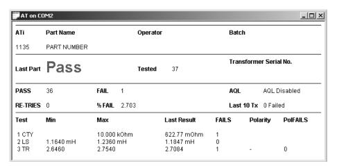
The batch statistics window display is automatically shown once this feature is enabled. For each AT connected to the Server the following information is displayed:
